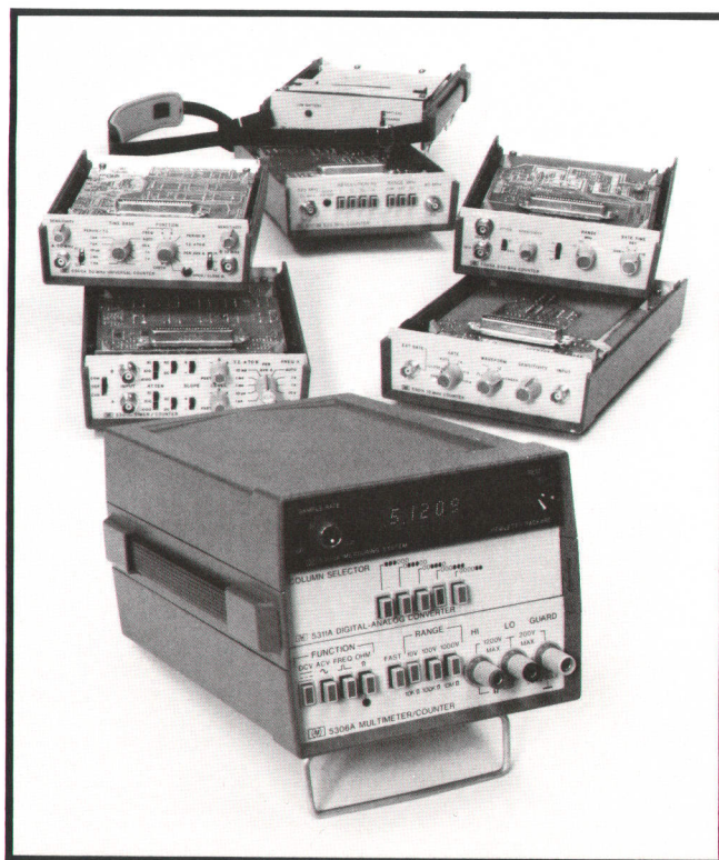
Fig. 1. Two new modules for the 5300 Measuring System are Model 5306A Multimeter/Counter (bottom module of instrument in foreground) and Model 5311A Digital-to-Analog Converter (center module). The Multimeter/Counter measures dc voltage, ac voltage, resistance, and frequency. Other elements of the system are the mainframe (top module), four counter/timer modules and a battery pack.
